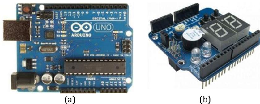
Gambar 1. Modul piranti: (a) Arduino Uno R3, (b) EMS *Basic I/O Shield*
